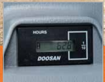
Hour meter (from ground level)
