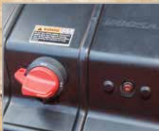
Battery cut-off switch
