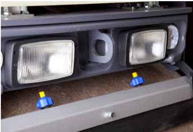
Pressurized sprinkler system with a powerful water pump and with self draining sprinkler tubes and nozzles.
